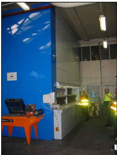
Photographs 7– Prevon Vertical Carousel (example of good practice) utilised by Victoria Police
